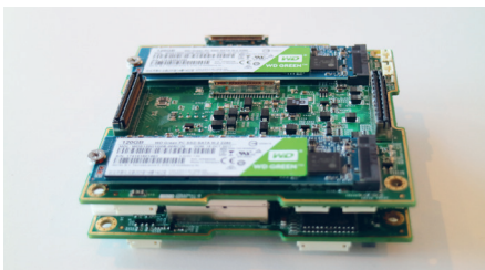
Side side view of DD-iX5 without casing showing top side iX5-EXT-100 extension interface board with M.2 SATA.
