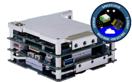
Unibap SpaceCloud iX5 Flight Model photographs for the D-Orbit Wild RIDE ION mission in Q2 2021.
