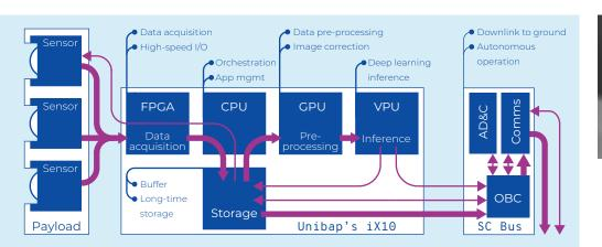
Application example Real time SAR-focusing, in-space edge computing to allow deep learning inference, compression and image proccessing in orbit.
